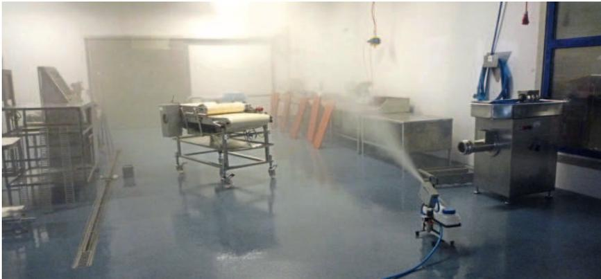
The ValloFog 3D cold fogging system kills nearly all microorganisms on a lasting basis.
