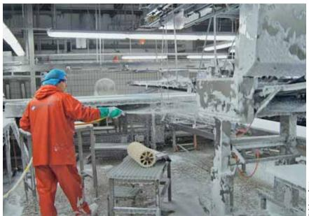
When cleaning slaughterhouses, a combination of dry ice jet cleaning, foam cleaning and high-pressure cleaning is normally used.
