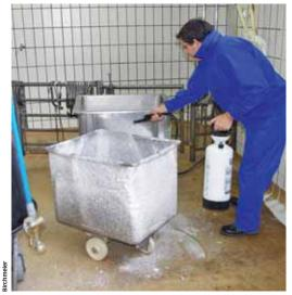
The portable Foam-Matic 5P foaming device creates a very dry, long-lasting foam without additional compressed air. It can be used in many situations and simplifies the cleaning of butcher shop equipment.
