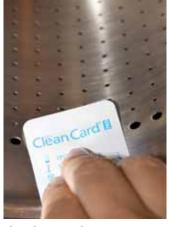
The Clean Card PRO test verifies correct cleaning in seconds.
