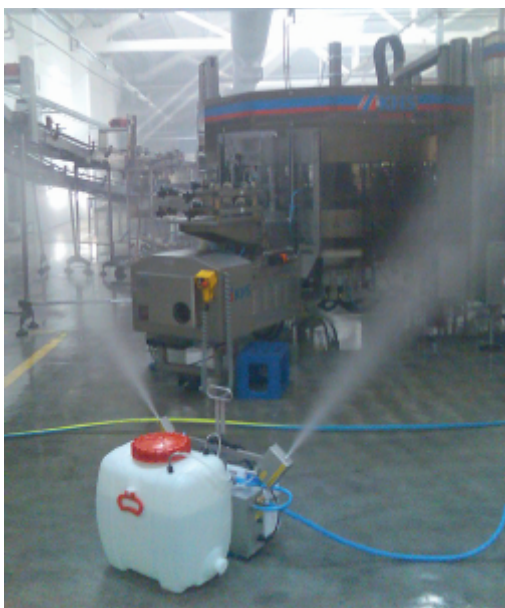
A fast, long-lasting preventive cold aerosol procedure provides effective sterilization of air as well as surfaces in production companies.
